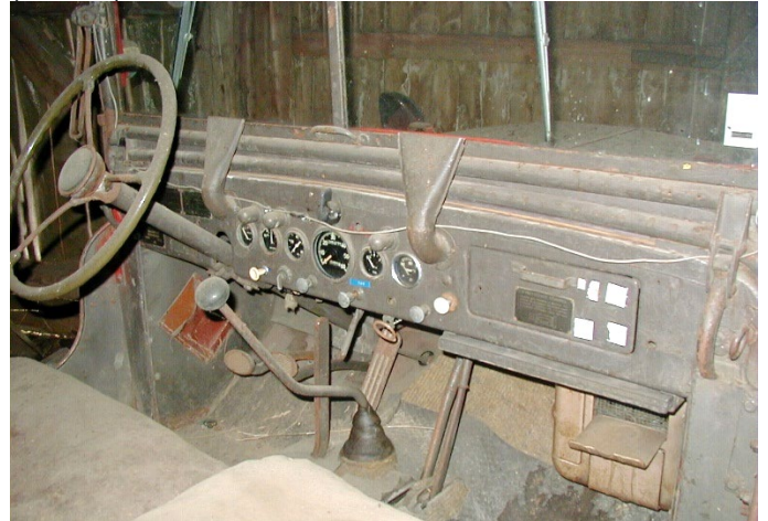
Interior view of the dash – with the Swedish data plates, different gauges, and heater blower flutes pointed at the windshield. (2007)
