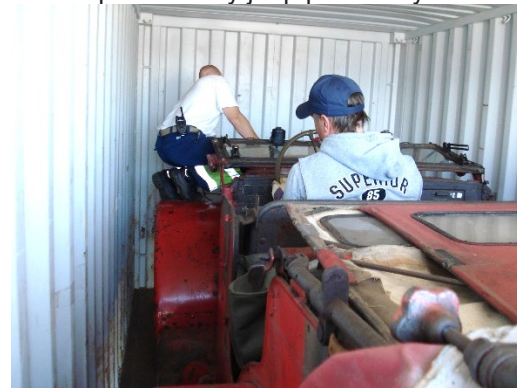
Pulling it up to the wall of the shipping container, before blocking in the wheels and axles with dunnage prior to sealing up the container – July 24, 2008.
